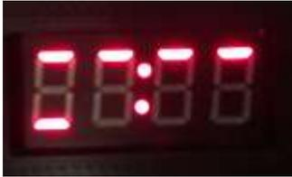
Here the Gate Length is 4 (the maximum), as shown by the 4 bars at the top, and the Step Repeat is 1 (the minimum), as shown by the 1 bar at the bottom.
